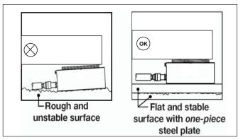
Figure 3: Cylinder Base Support
