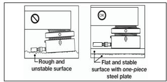
Figure 3, Cylinder Base Support (typical)
