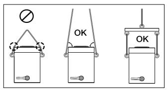
Figure 2, Lifting Arrangements (typical)
