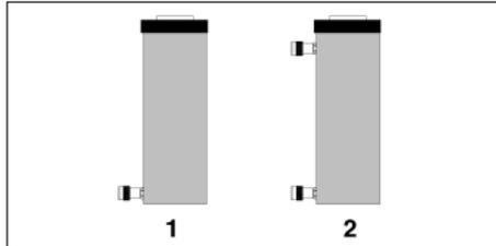
**IMPORTANT:** Double-acting cylinders must have both couplers connected.
