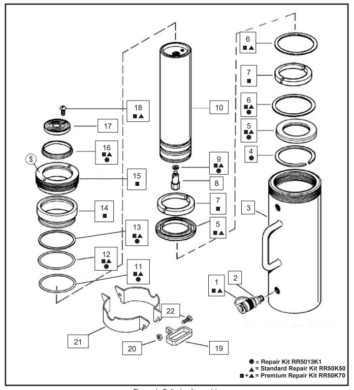
Figure 1: Cylinder Assembly
